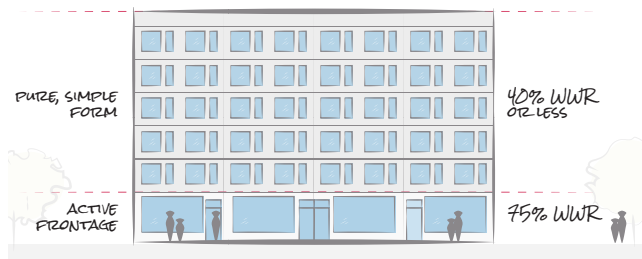
While retaining at-grade transparency, targeting lower window-to-wall ratios on building elevations can significantly reduce energy demand.
